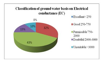
Figure.4 Classification of Ground Water Based on Electrical Conductance (EC)
